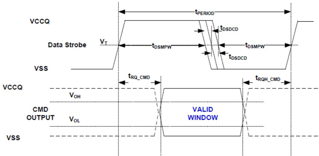
Note:  $V_T = 50\%$  of  $V_{CCQ}$ , indicates clock reference point for timing measurements.
