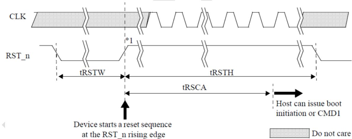
\*1: Device will detect the rising edge of RST\_n signal to trigger internal reset sequence
