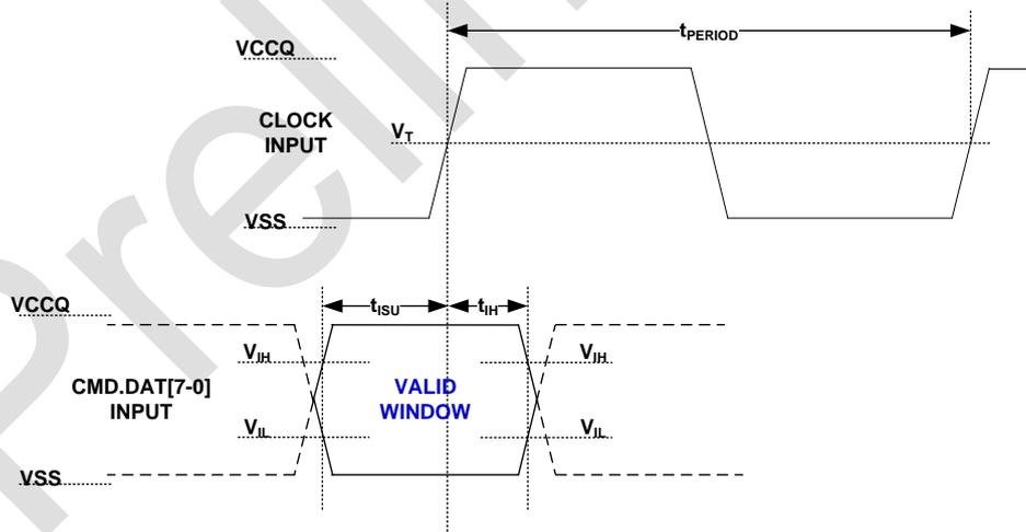
Note 1:  $t_{ISU}$  and  $t_{IH}$  are measured at  $V_{IL}(\text{Max})$  and  $V_{IH}(\text{Min})$ .
