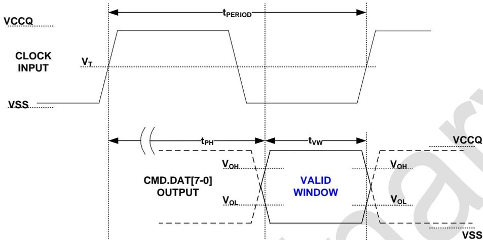
Note:  $V_{OH}$  denotes  $V_{OH}(\text{Min})$  and  $V_{OL}$  denotes  $V_{OL}(\text{Max})$ .
