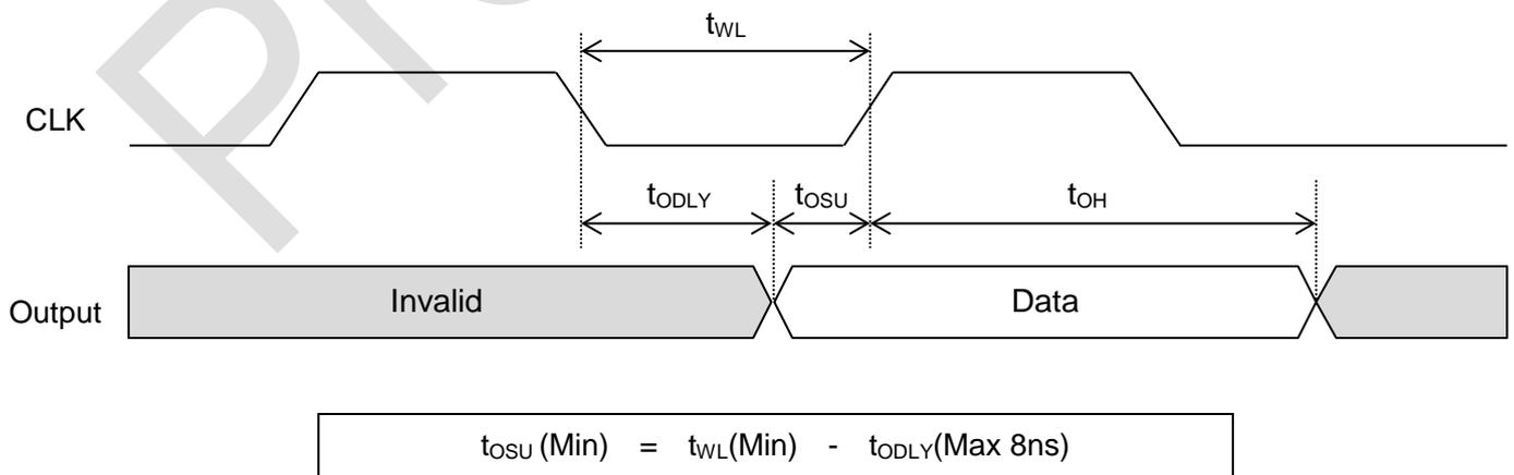
**Figure 2 Output timing**
