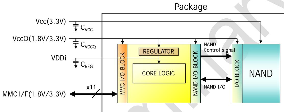
Figure 1 THGBMJG7C2LBAU8 Block Diagram
