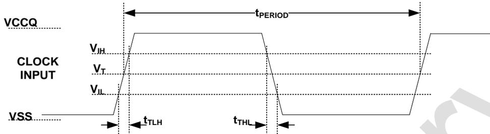
Note 1:  $V_{IH}$  denote  $V_{IH}(\text{Min})$  and  $V_{IL}$  denotes  $V_{IL}(\text{Max})$ .
